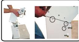
STEP 5: Slide the top portion of the control box into the lower portion. Secure on each side with (3) screws and lock washers.
