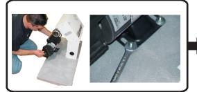
STEP 6: Place the pump over the (4) mounting bolts, install nuts and washers and leave slightly loose until header assy is aligned.
